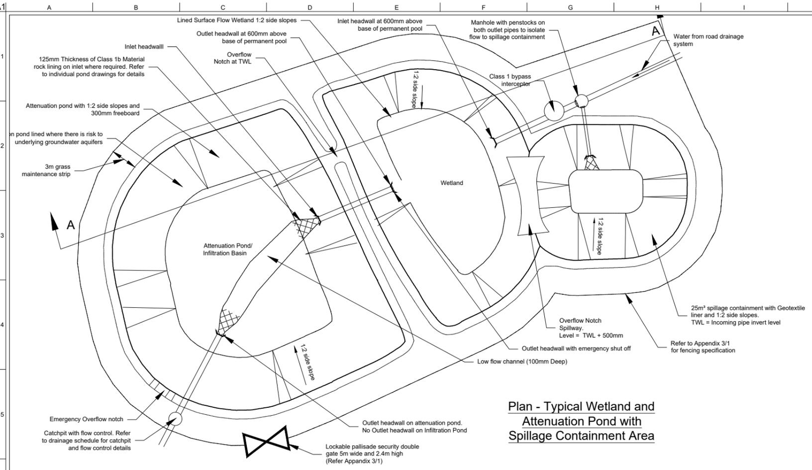
**Plan - Typical Wetland and Attenuation Pond with Spillage Containment Area**
